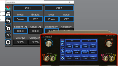
Control SLICE through the front panel, a GUI, or serial commands
