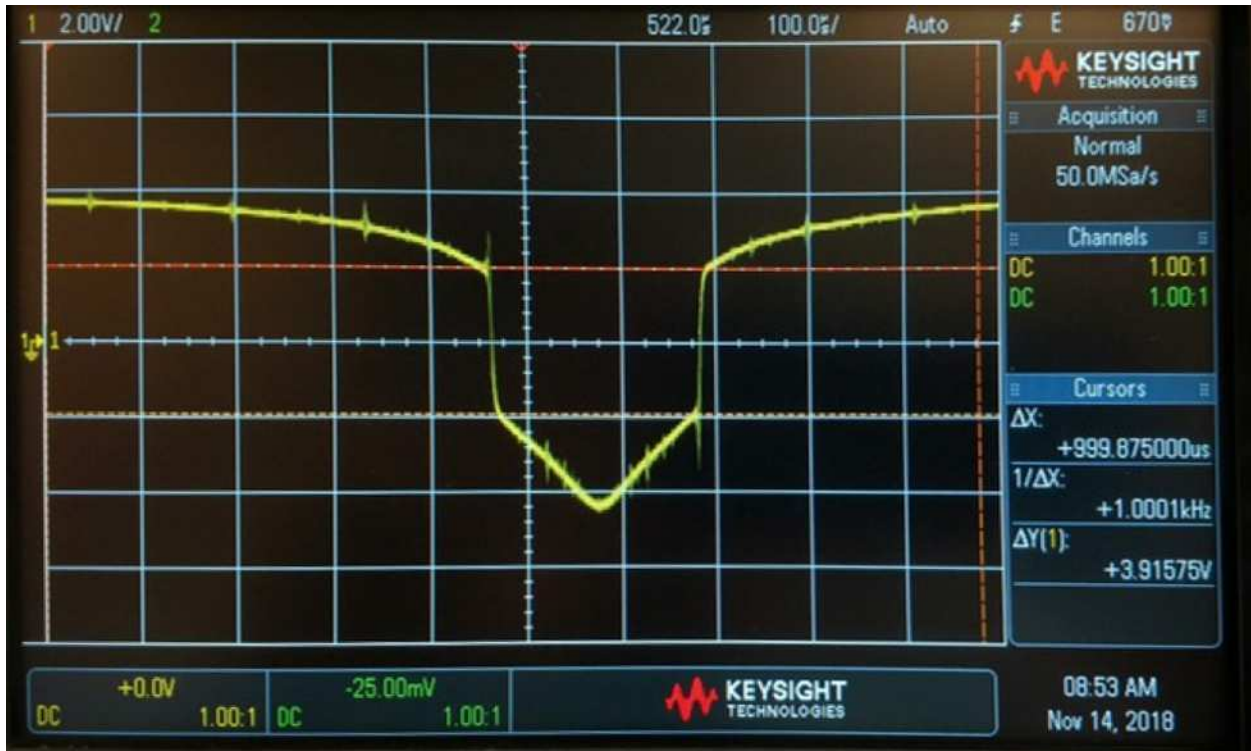
Figure 2. Oscilloscope trace showing the unlocked error signal. The regions on the trace with the largest slope are where the PFD is performing as a phase detector.
