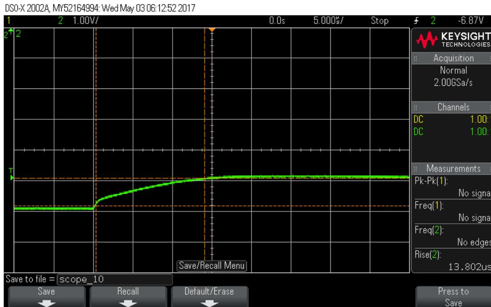
**Figure 4. Oscilloscope capture of timing to catch lock**
