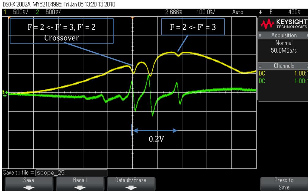
Figure 2. Portion of the D2 spectrum of Rb used in experiment. DC error signal (yellow) and demodulated FM error signal (green).
