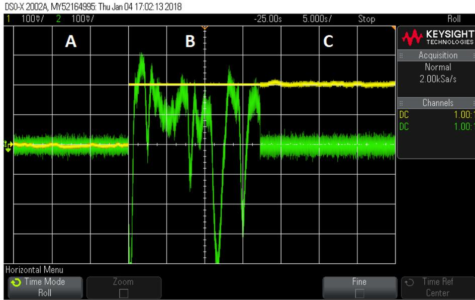
**Figure 3. Oscilloscope traces in “roll” mode showing Servo Output (yellow) and DC Error Input (green). Section A: System initially locked to the  $F=2 \leftarrow F'=3$ ,  $F'=2$  Crossover transition. Section B: System free-running with Servo Out held to a controlled value near the center of the  $F=2 \leftarrow F'=3$  transition. Section C: System set to lock state at new lock point.**
