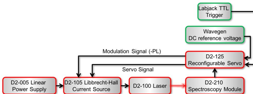
Figure 1. Experimental Configuration.
