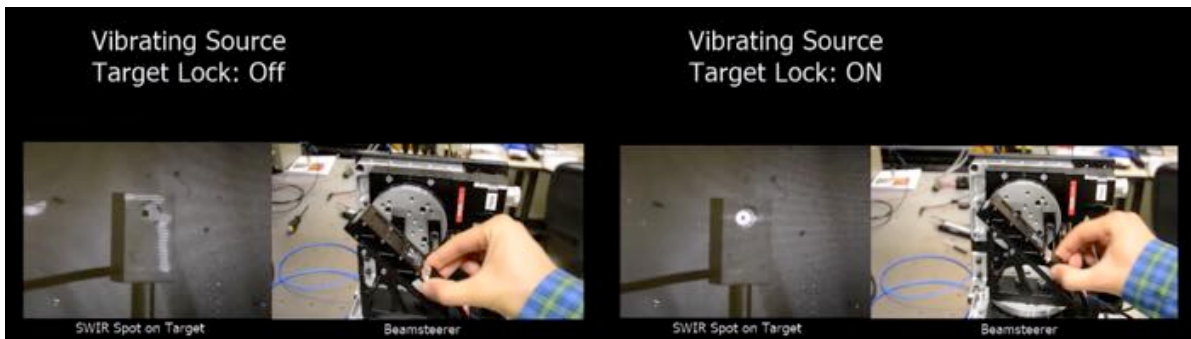
Figure 7: Demonstration of servo or target locking the EO beamsteerer to compensate for a vibrating source.
