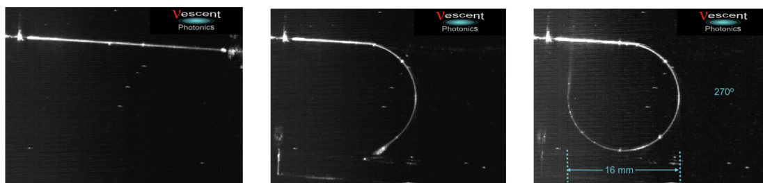
Figure 3. Example data from an electrode pattern that provided steering of 1550nm light by 270° in a package smaller than the size of a US dime.
