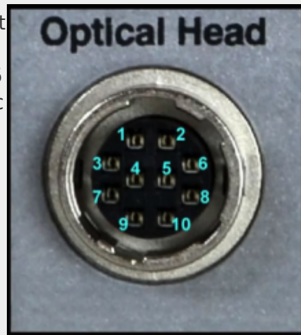
Fig. 4: Pin-Out for the LC-105 connection to the optical head.
