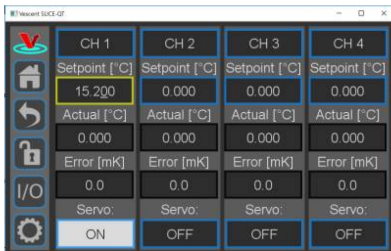
Fig. 18: Knob adjustment of Temperature setpoint for CH 1
