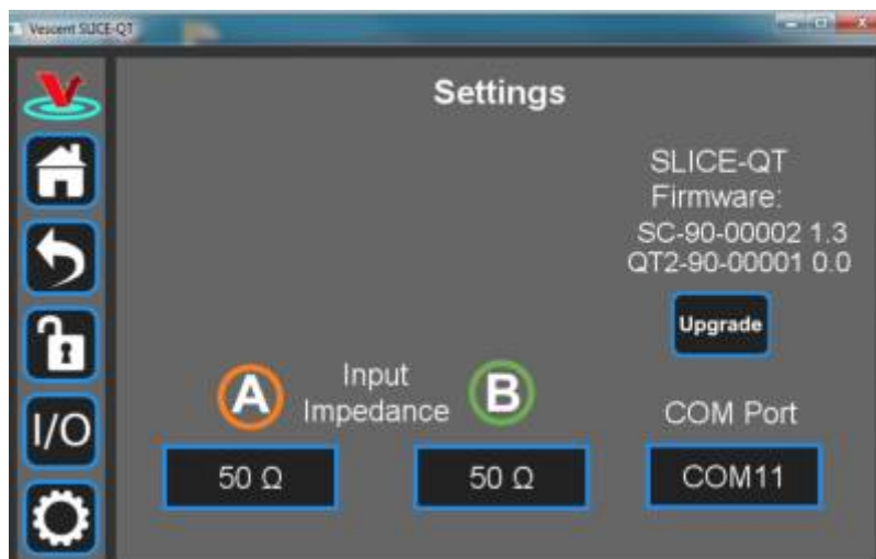
Fig. 42: User-programmable system settings from host GUI
