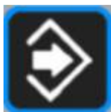
Fig. 16: Enter button Accepts edits and exits keypad.
