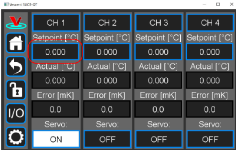
Fig. 17: Select Temperature setpoint for CH 1
