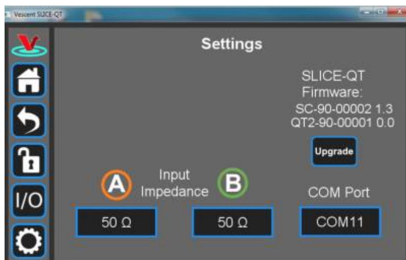
Fig. 42: User-programmable system settings from host GUI
