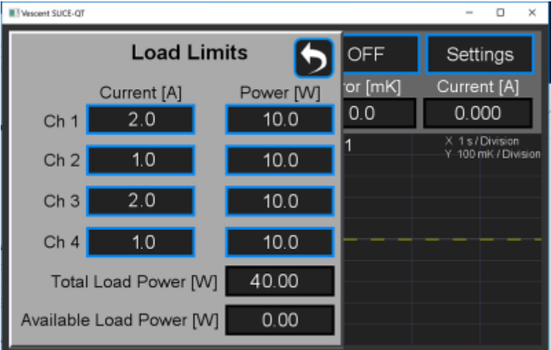
Fig. 25: Screen for adjustment of control power capacity
