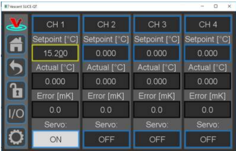
Fig. 18: Knob adjustment of Temperature setpoint for CH 1
