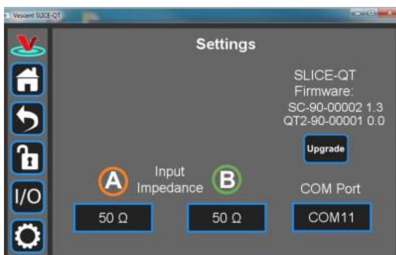
Fig. 42: User-programmable system settings from host GUI
