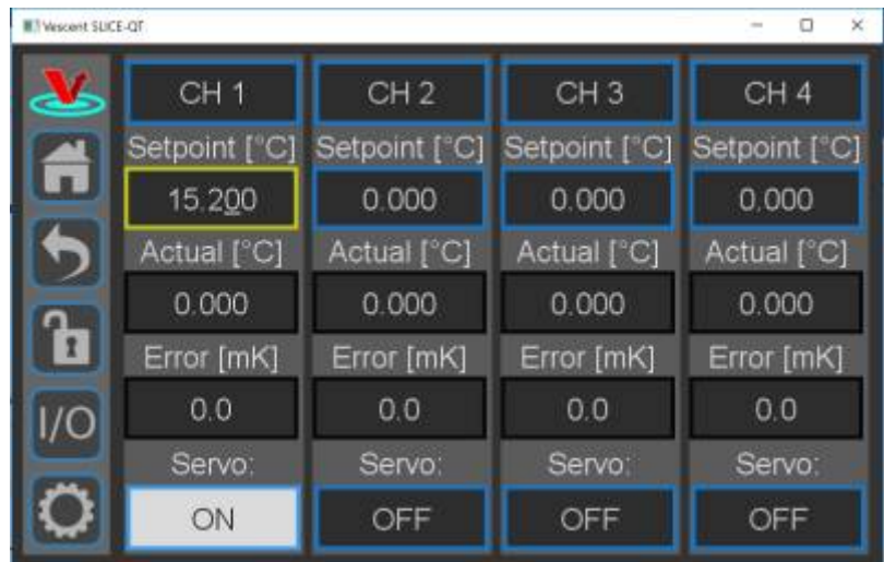
Fig. 18: Knob adjustment of Temperature setpoint for CH 1
