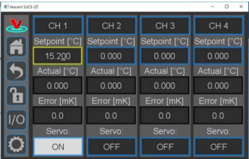
Fig. 18: Knob adjustment of Temperature setpoint for CH 1
