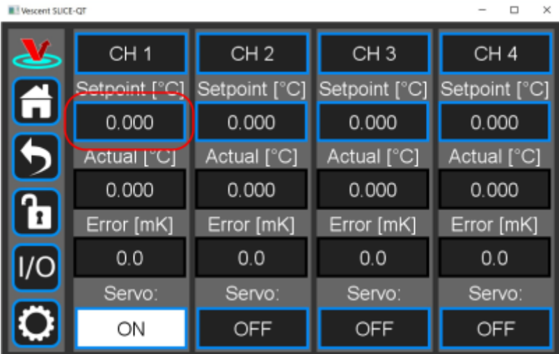
Fig. 17: Select Temperature setpoint for CH 1
