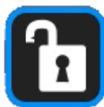
Fig. 9: Lock button (shown in unlocked mode) Locks out further modification of parameters. Touch to lock or unlock parameter entry. It is still possible to engage the temperature control loops when system is locked, but it is not possible to change the set point temperature or loop parameters, etc.
