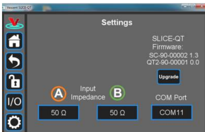
Fig. 42: User-programmable system settings from host GUI
