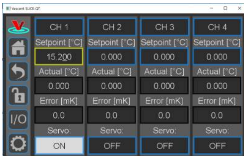
Fig. 18: Knob adjustment of Temperature setpoint for CH 1
