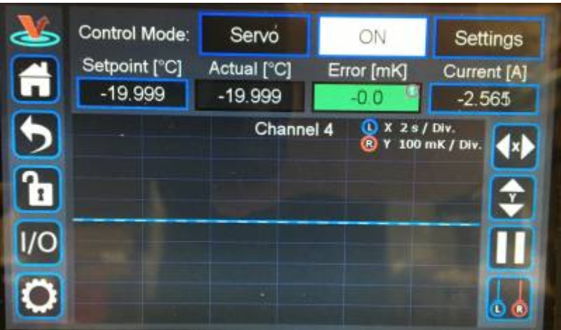
Fig. 34: CH 4 \Delta T data is being delivered to front-panel I/O channel 1
