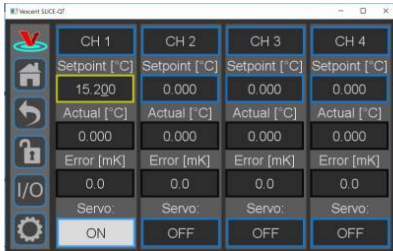
Fig. 18: Knob adjustment of Temperature setpoint for CH 1
