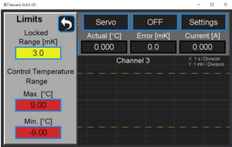
Fig. 24: Screen for setting absolute extrema and lock range
