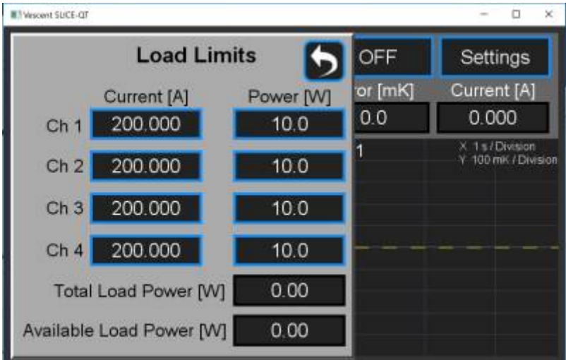
Fig. 25: Screen for adjustment of control power capacity
