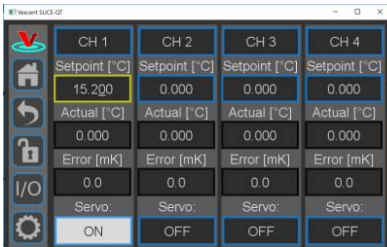
Fig. 18: Knob adjustment of Temperature setpoint for CH 1
