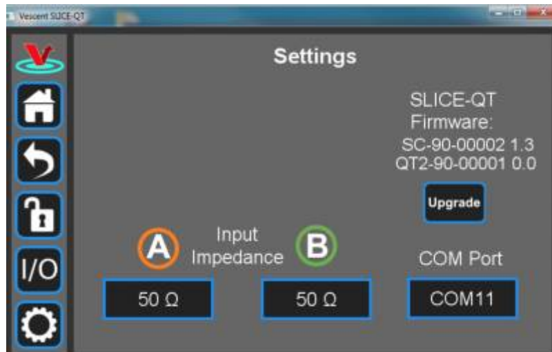
Fig. 42: User-programmable system settings from host GUI
