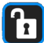
Fig. 9: Lock button (shown in unlocked mode) Locks out further modification of parameters. Touch to lock or unlock parameter entry. It is still possible to engage the temperature control loops when system is locked, but it is not possible to change the set point temperature or loop parameters, etc.
