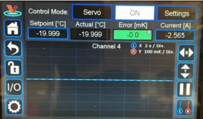
Fig. 34: CH 4 ΔT data is being delivered to front-panel I/O channel 1
