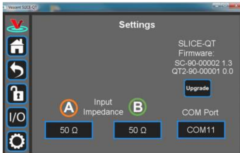
Fig. 42: User-programmable system settings from host GUI
