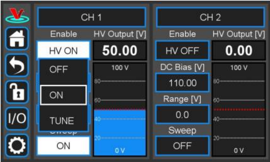
Fig. 20: Controlling the internal ramp
