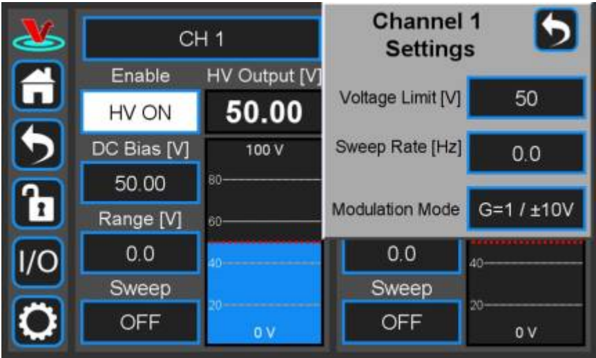
Fig. 18: Setting parameters of individual channel
