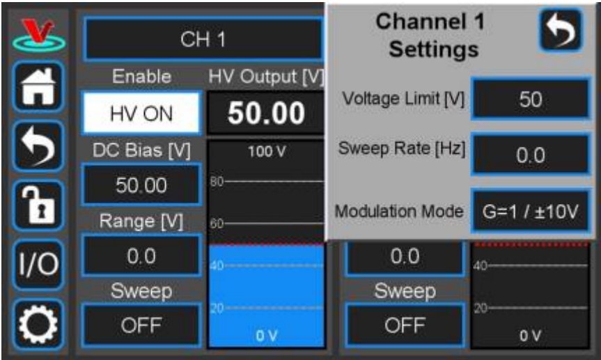
Fig. 18: Setting parameters of individual channel
