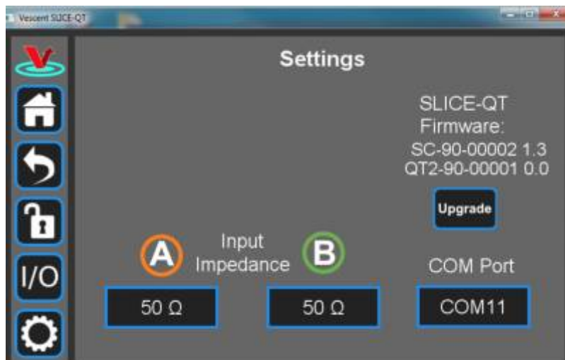
Fig. 35: User-programmable system settings from host GUI
