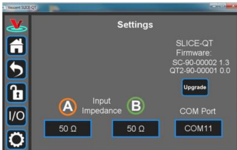
Fig. 35: User-programmable system settings from host GUI
