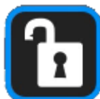
Fig. 7: Lock button (shown in unlocked mode) Locks out further modification of parameters. Touch to lock or unlock parameter entry. When in lock mode, it is still possible to toggle the current on and off, but it will not be possible to change the set point or other operation parameters.
