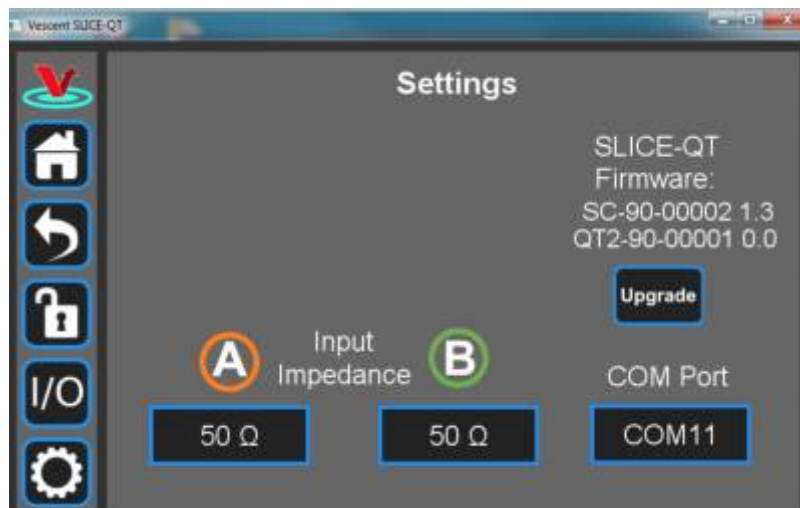
Fig. 35: User-programmable system settings from host GUI
