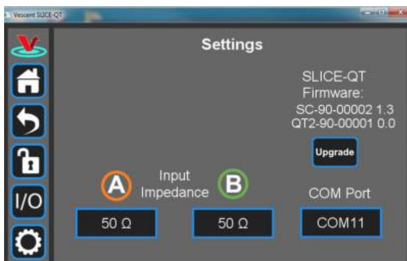
Fig. 35: User-programmable system settings from host GUI
