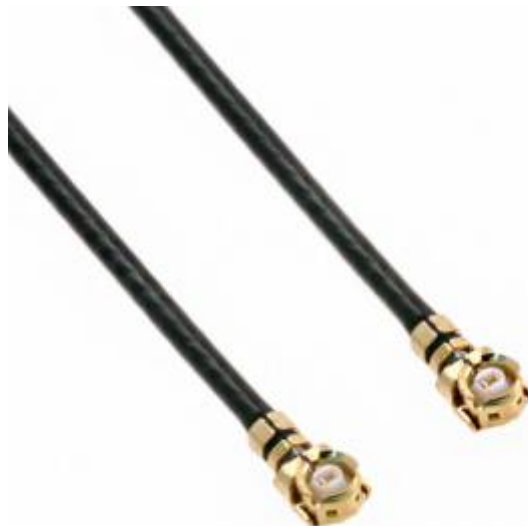
Fig. 7: Surface mount UMCC connector. Molex PN: 0734120110
