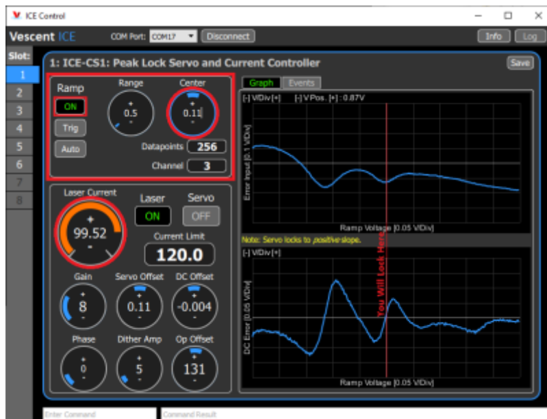
Fig. 11: CS1 GUI showing the Ramp Box, and the Center Line to which the Servo Locks
