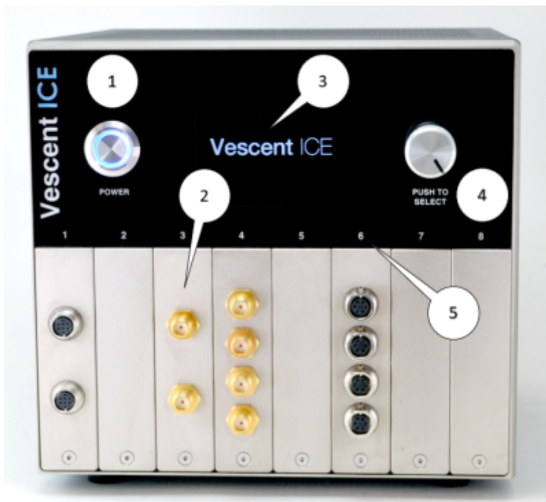
Fig. 14: Front Panel of the ICE Box
