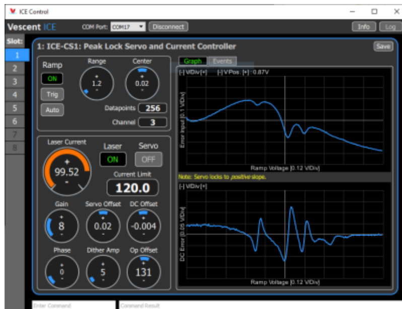
Fig. 10: Rb Spectroscopy (top) and Peak Lock Differential signal (bottom)
