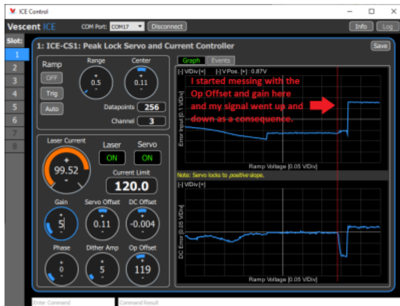
Fig. 13: Demonstration of how incorrect Offset and Gain can affect your lock
