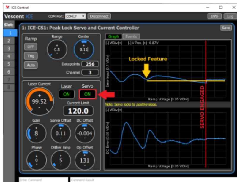
Fig. 12: When the ICE Box locks to spectroscopy, the top graph will flatten out at a DC offset corresponding to the locked feature (Yellow Line)
