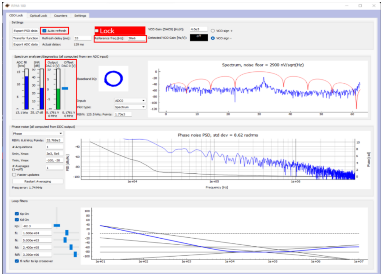
Fig. 9: Centering f(\text{CEO}) on reference frequency (Baseband IQ optimization)
