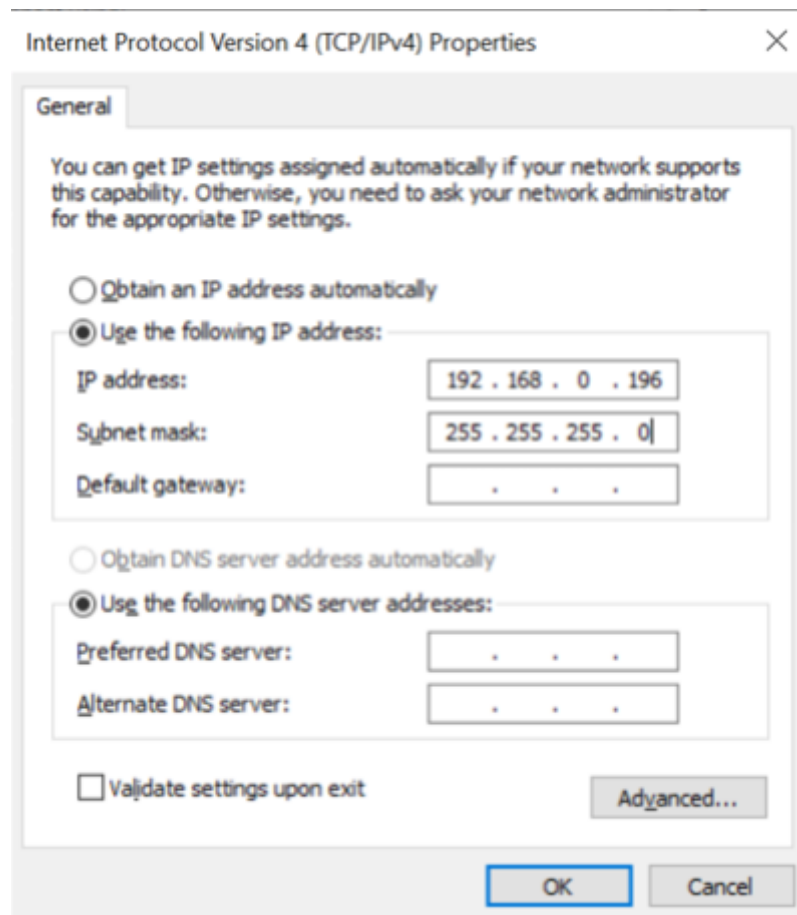
Fig. 14: The IPv4 Properties page, with the IP Address and Subnet Mask filled in.
