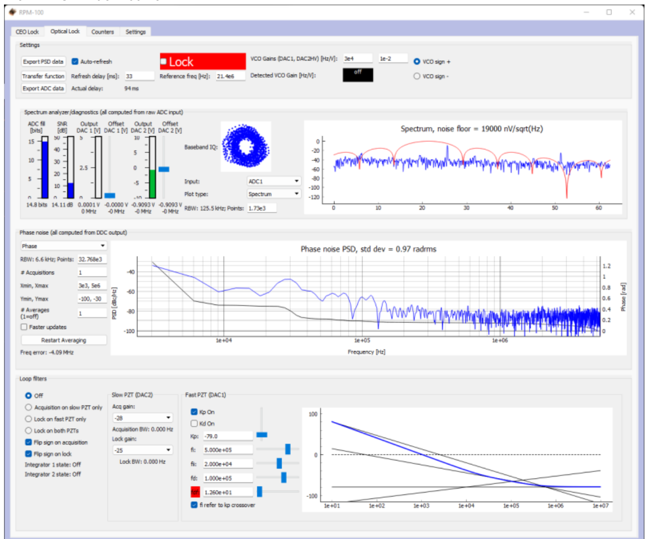
Fig. 11: Centering f_{\text{opt}} on reference frequency (Baseband IQ optimization)
