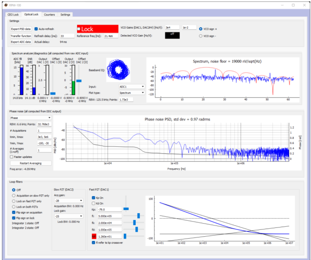
Fig. 7: Centering f_{\text{opt}} on reference frequency (Baseband IQ optimization)
