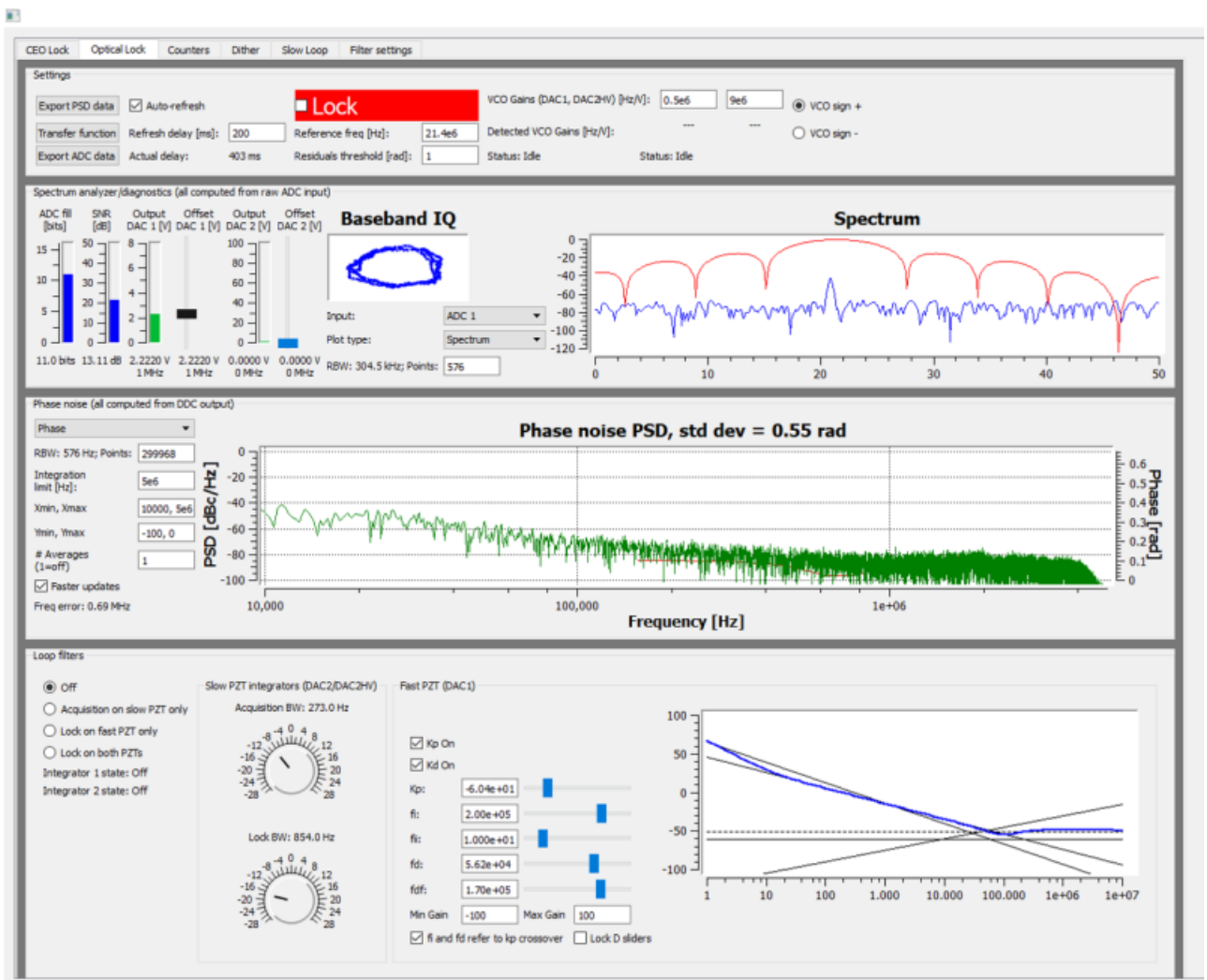
Fig. 7: Centering f_{opt} on reference frequency (Baseband IQ optimization)
