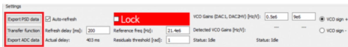
Fig. 9: Export ADC data, or the Phase noise PSD chart to CSV
