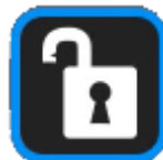
Fig. 7: Lock button (shown in unlocked mode) Locks out further modification of parameters. Touch to lock or unlock parameter entry. There are some parameters with values which can be changed while the system is locked, such as the PZT range, but in general parameters which control a state or value, such as the set point temperature of a pump diode, cannot.
