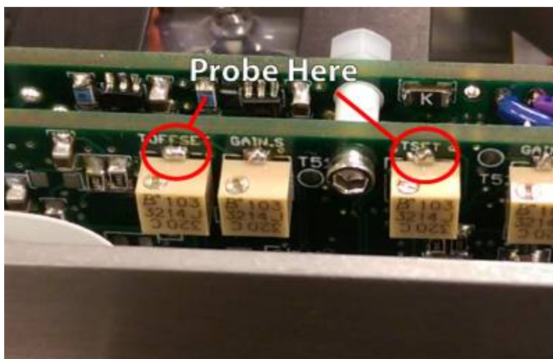
Fig. 4: Locations to probe with voltmeter while adjusting trimpots.
