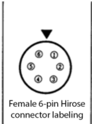
Fig. 2: Pin numbering on female Hirose 6-pin connector
