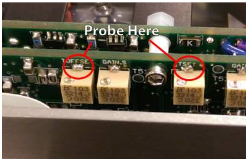
Fig. 4: Locations to probe with voltmeter while settings while adjusting trimpots.
