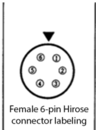
Fig. 3: Pin numbering on female Hirose 6-pin connector
