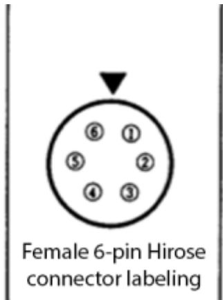
Fig. 3: Pin numbering on female Hirose 6-pin connector
