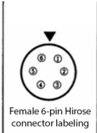
Fig. 3: Pin numbering on female Hirose 6-pin connector
