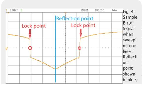
The reflection point on the Error Signal is where the two lasers are at the same frequency. The Error Signal is a even function of offset frequency (Error( $\Delta f$ ) = Error(- $\Delta f$ )), so there is a reflection point about  $\Delta f$ =0. The sharp slope to the left or right of the  $\Delta f$ =0 point is the lock point and can be adjusted by changing the VCO frequency. Which of the two lock points the laser will lock to will
