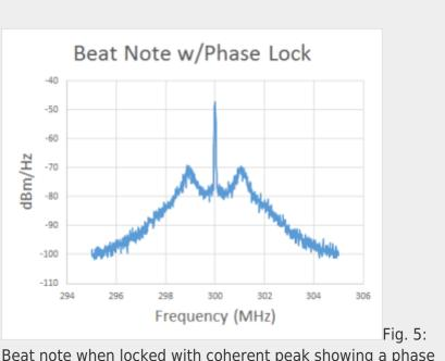
Beat note when locked with coherent peak showing a phase lock.
