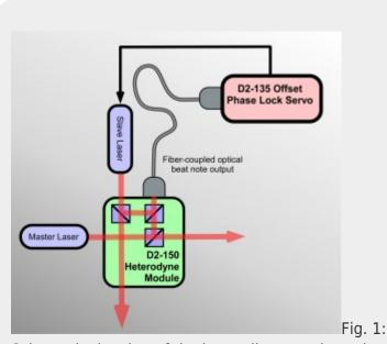
Schematic drawing of the laser alignment in to the D2-150 Heterodyne Module.
