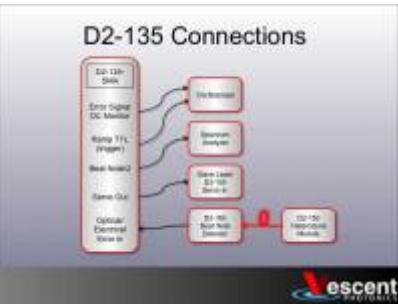
Fig. 3: Initial electrical connections to D2-135. (As shown for D2-135-SMA. For D2-135-FC, connect optical output of D2-150 directly to SC fiber input on face of D2-135.)
