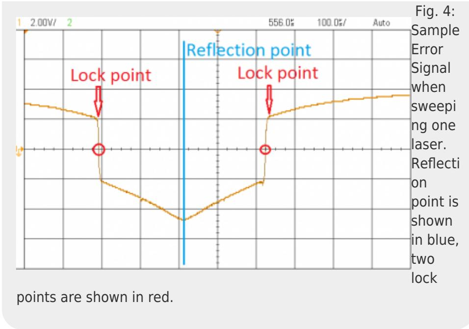
Fig. 4: Sample Error Signal when sweeping one laser. Reflection point is shown in blue, two lock
