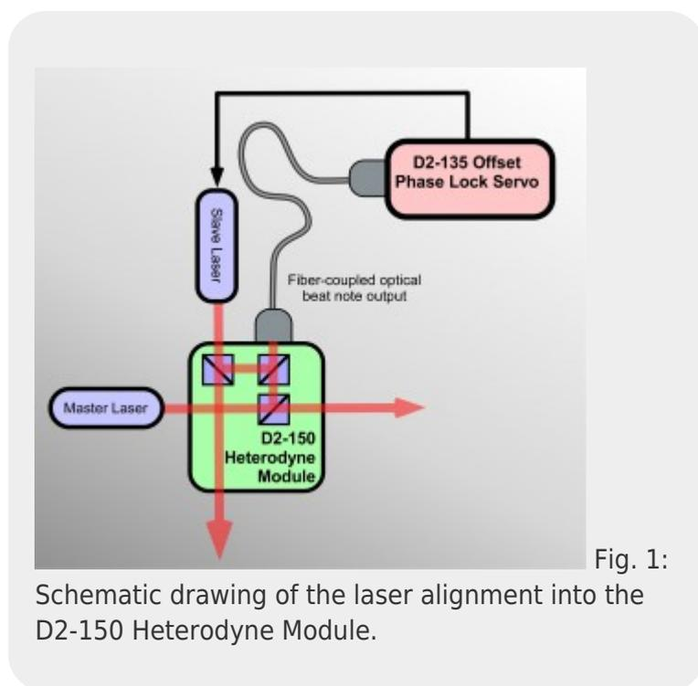
Place the two lasers and the D2-150 or D2-250 as shown in either [figure 1](#) or [figure 2](#) depending on which unit you are using: the two lasers oriented 90° relative to each other and both pointing at the
