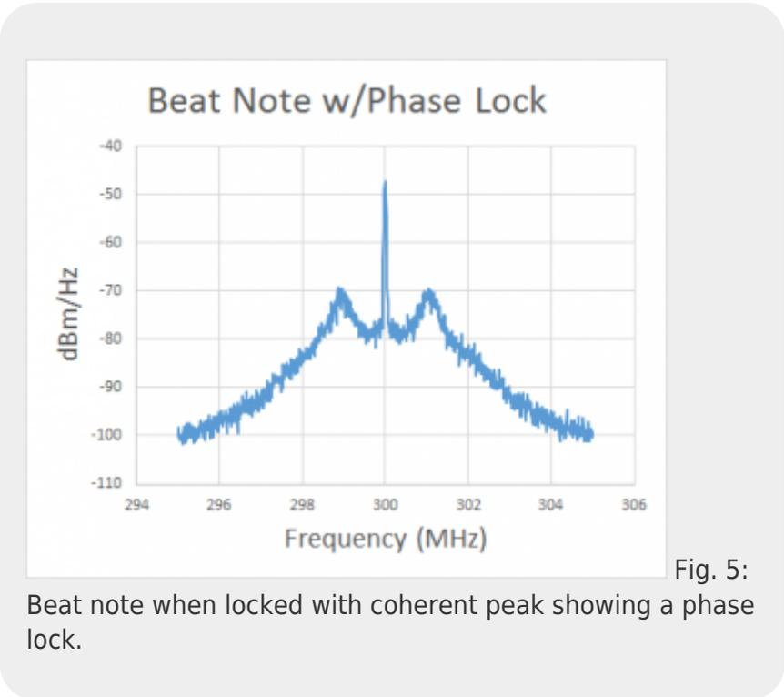
Fig. 5: Beat note when locked with coherent peak showing a phase lock.
