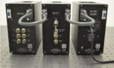
D2 Electronics with new-style power distribution cables (back view)
